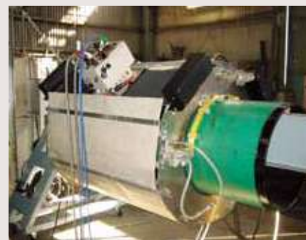
Auto lining device for thermal-contraction tube
