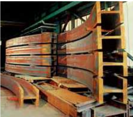
H-steel for bridge pier
