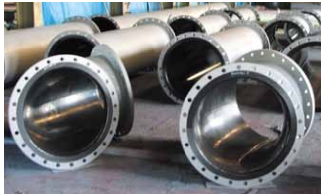
Polyethylene lining pipe (inside)
