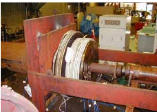
Shrink fitting and thermal withdrawal
