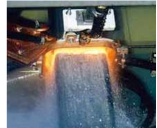
Pipe wall thickening
