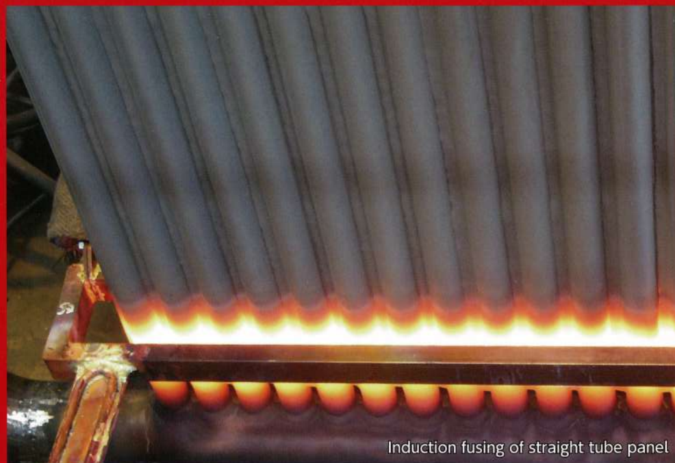
Panel undergoing simultaneous fusing and bending
