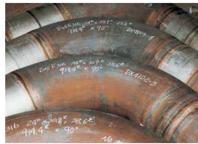
1.5DR BENDS for Nuclear power plant ASTM A312 TP316L 24" X 38.6mm X 914.4mmR
