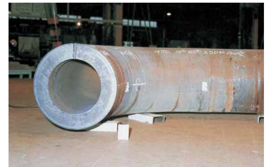
1.5DR BENDS for Thermal power plant ASTM A106 18" X 82mmT X 685.8mmR
