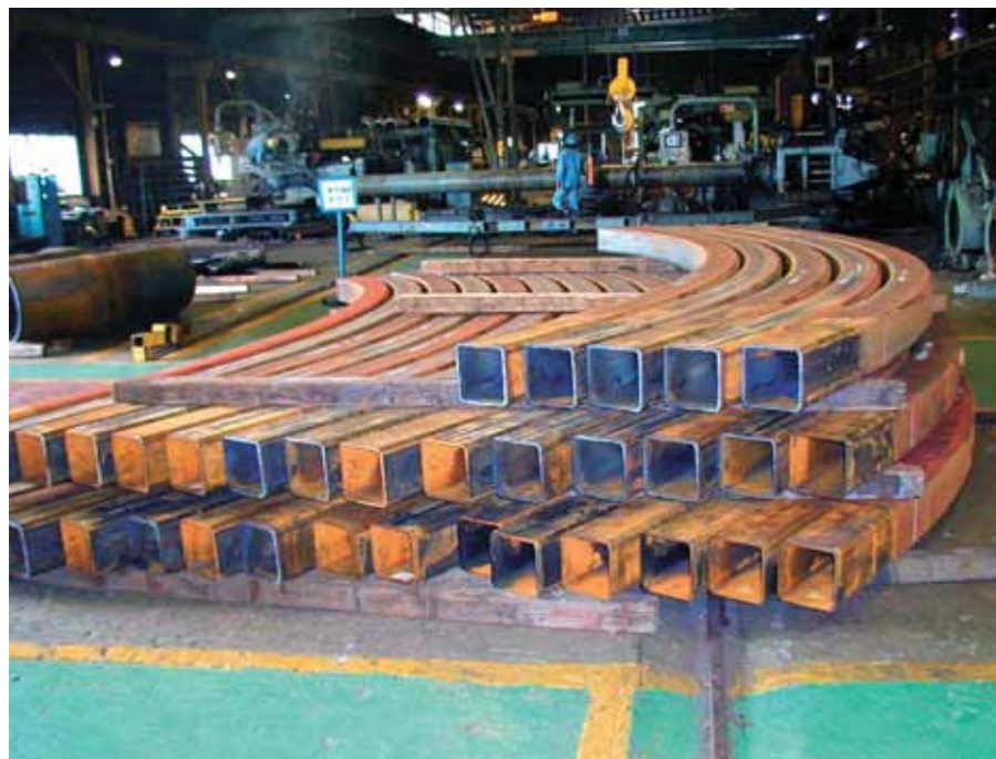
Square Pipe 200×200m 9.0mm-thickness
