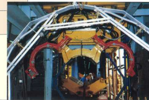
鋼管溶接部焼鈍装置 Post-weld annealer of pipes
