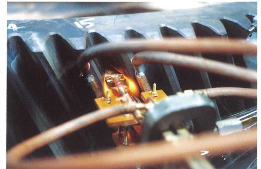
歯車の移動焼入れ Progressive hardening of gear tooth
